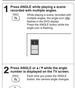
You can change the camera angle directly by pressing the number buttons corresponding to its angle number instead of using the  $\blacktriangle / \checkmark$  buttons.
